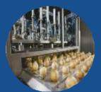
Transformation and valorization of onions into ready-to-use packaged products, sliced or powdered, for use in culinary preparations. The manufacturing process includes peeling/cutting, even drying grinding and packaging
